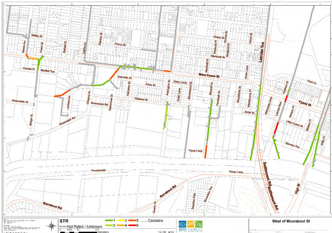
Figure 3.4 Western study area (Shannon Avenue - Moorabool Street) STR grading
