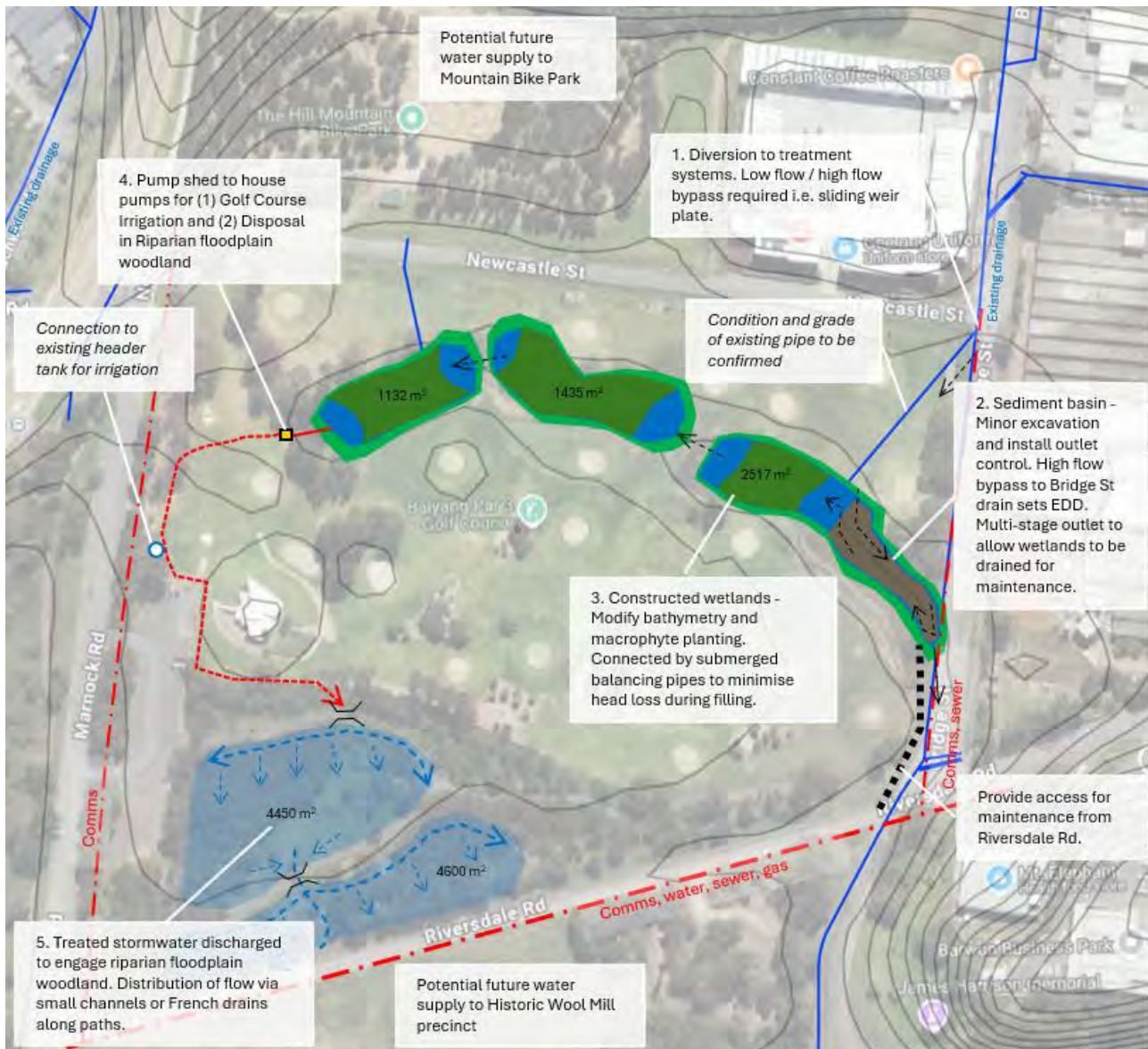
Figure 8.4 Proposed constructed wetlands and stormwater harvesting concept
