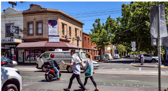
Brunswick Street, Fitzroy Raised Thresholds at street intersection improves pedestrian visibility and safety whilst slowing vehicles without changing the right of way. Photo credit: Melissa & Chris Bruntlett, modacitylife
