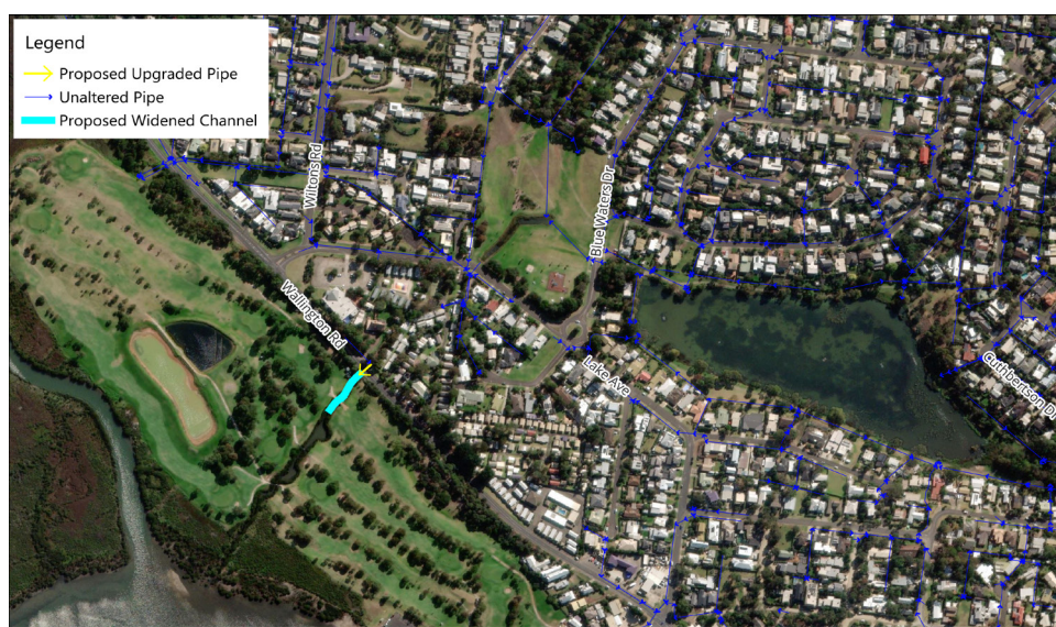
Figure 4: Wallington Road Culvert Upgrade.
